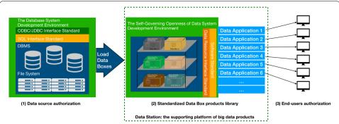
**Fig. 1** The supporting system of big data products based on Data Box. Firstly, the platform gets authorization from data sources and load data into Data Boxes. Then the data station stores standardized Data Boxes and serves data applications with proper standards, which are finally provided to end-users through authorization
