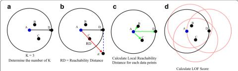
**Fig. 3** The illustration of Local Outlier Factor (LOF) process. **A** Determine the number of k-value **B** calculate the Reachability Distance (RD) **C** Calculate the Local Reachability Distance (LRD) **D** Calculate the LOF Score for each data points
