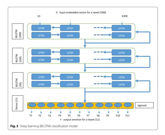
corresponding to the 11 emotions. The activation is a sigmoid function; it gives a probability of each emotion. We approximate the values to 0, 1 class for each 11 output representing the 11 emotions. Fig. 3 shows the network structure.
