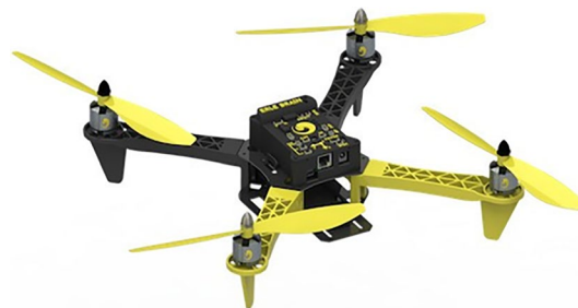
Fig. 1 We use drone from Erle Robotics [11] based on the ROS for delivering items. Erle-copter’s flight time is around 20 min with a 5000 mAh battery, and the drone is built to support a payload of up to 1 kg
