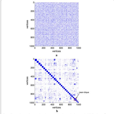
**Fig. 6** Clique ordering is shown on the right compared to the initial ordering on the left. The dense off diagonal blocks reveal large cliques along the diagonal that are tightly connected and form much larger *near-cliques*. **a** Initial ordering. **b** Clique ordering
