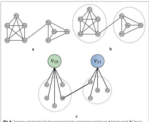
**Fig. 4** Overview and intuition for the proposed graph compression techniques. **a** Simple graph. **b** Cliques identified. **c** Encoding Intuition
