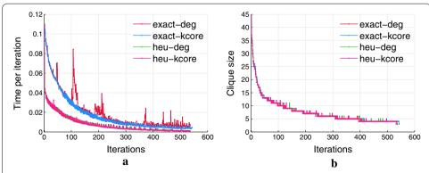
**Fig. 5** Four variants of GraphZIP are compared. Runtime decreases with clique size as a result of the search space shrinking after each clique is found and removed from the graph. Further, the heuristic is 2-3 times faster than the exact clique finder. **a** Time. **b** Clique size
