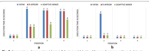
**Fig. 8** Comparision of conventional Apriori, R-Apriori and Adaptive-Miner performance. **a** Kosarak dataset min sup = 0.60%. **b** BMSWebView2 dataset min sup = 0.10%
