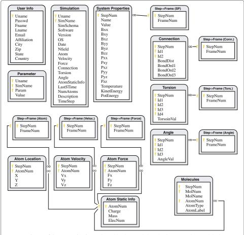
**Figure 3 Schema of the DCMS database.** The golden key symbol marks the primary keys and the lines represent foreign keys. Note that there exist foreign keys from all lds in tables *Connection, Torsion*, and *Angle* to the *Atom Static Info* table. We did not draw them due to space limit.
