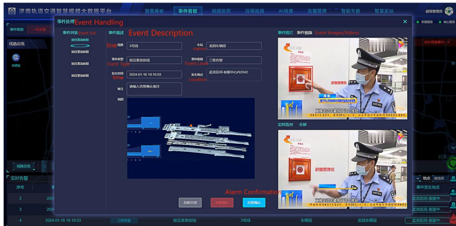
Fig. 21 The alarm prompt of the platform can display the description of the alarm event, so as to facilitate the operation personnel to grasp what abnormal events occur in where
