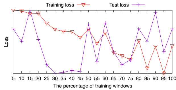
Fig. 4 The relationship between the training/test loss and the percentage of sliding windows for training
