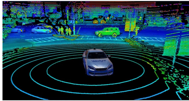
Fig. 4 Source – Velodyne. This image shows a 3D map of the surroundings of an autonomous car, constructed using lidar sensor data. The map illustrates the precision and accuracy of the lidar sensor in capturing the geometry of the environment, including buildings, roads, and other obstacles. The use of lidar sensors in autonomous cars is crucial for creating a detailed and accurate map of the car's surroundings, which is then used for navigation and localization
