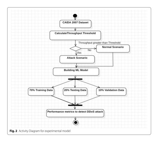
data is compared with the threshold. Throughput above the threshold is categorised as an attack, else normal. Later, the ML model such as logistic regression and naïve bayes is used to further validated the proposed model. The Median of the CAIDA 2007 Dataset is considered as the throughput threshold.
