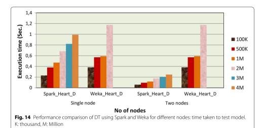
million, respectively, we can see that the total execution time decreases as the number of nodes increases. This indicates that the higher the number of nodes involved in computation, the faster the algorithm will be due to the distributed computing. In contrast, the execution time of standard DT using Weka with two nodes remains stable due to the undistributed computing.
