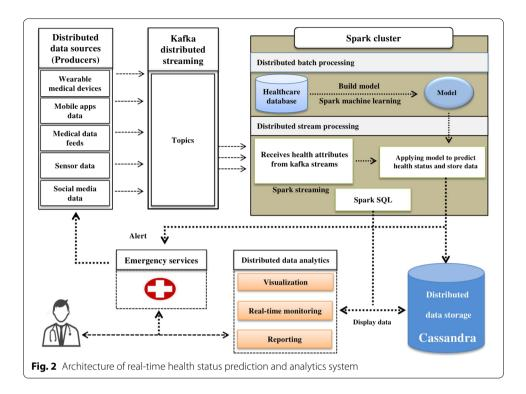
Using Apache Zeppelin the data will be retrieved from database and making dashboard that displays data in charts, lines and tables in real-time. Based on the proposed system architecture, data from monitors (IoT) can be analyzed in real-time and send an alert to care providers, so they know instantly about changes in a patient's condition. The data will be refreshed automatically by fixing times intervals. The following subsections give detailed flow.
