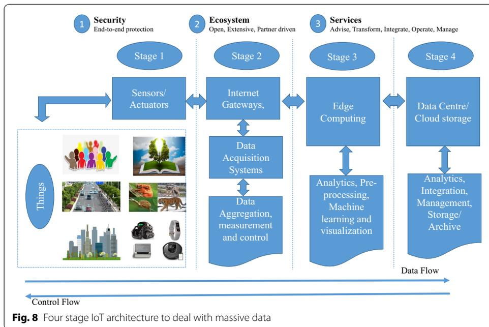
**Fig. 8** Four stage IoT architecture to deal with massive data
