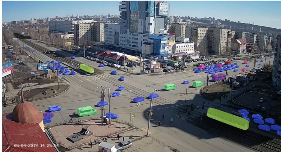
Fig. 1 Example of an image from our dataset. Blue, yellow, green, red, violet, pink and black polygons stands for the “car”, “tram”, “van”, “bus”, “trolleybus”, “truck” and “unlabeled” objects respectively
