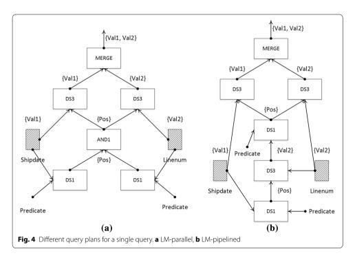
There are two possible execution plans. They are shown in Fig. 4 (the figure and query are adapted from the reference [74]). It is possible to perform on-line switching from plan depicted on the top to the plan on the bottom, if filtering Shipdate's column produces too many results. In this case, "AND1" operator should be substituted by a sequence of "DS3" and "DS1" operators. If filtering produces a low number of results, on-line switching in the opposite direction is also possible.
