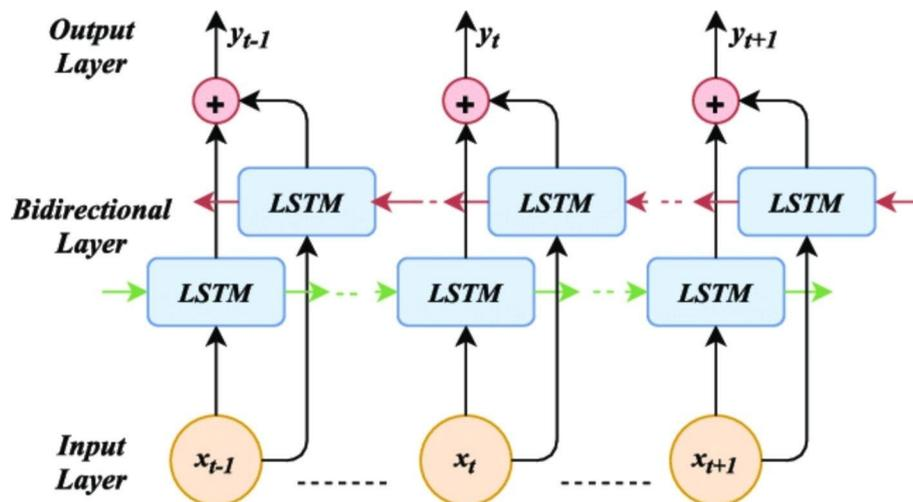
**Fig. 2** Bi-Directional LSTM Architecture
