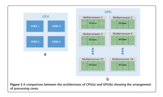
1000Tflops of processing power. This massive parallelism in GPU makes it a more appealing option for parallel computing applications.
